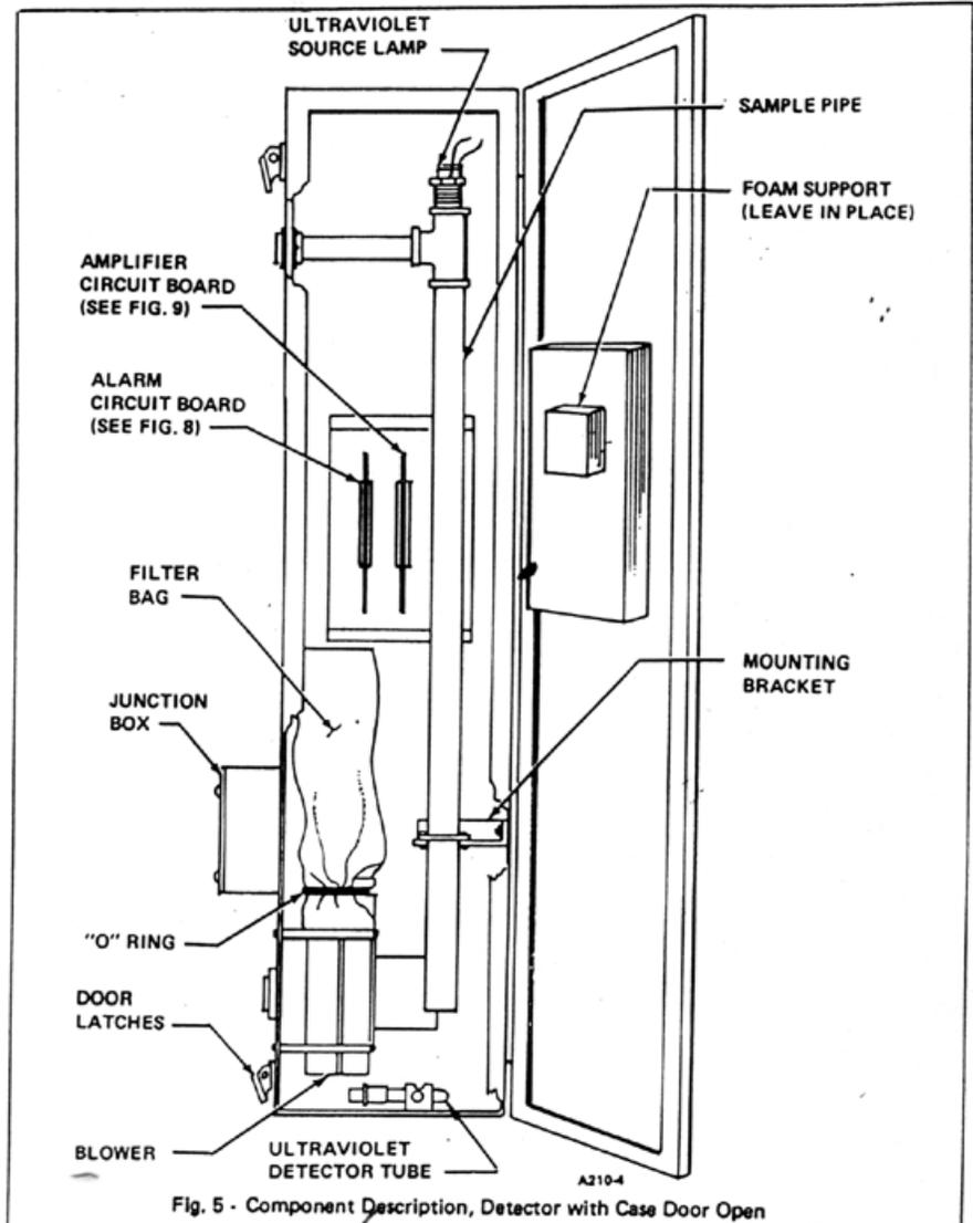
Fig. 5 - Component Description, Detector with Case Door Open
