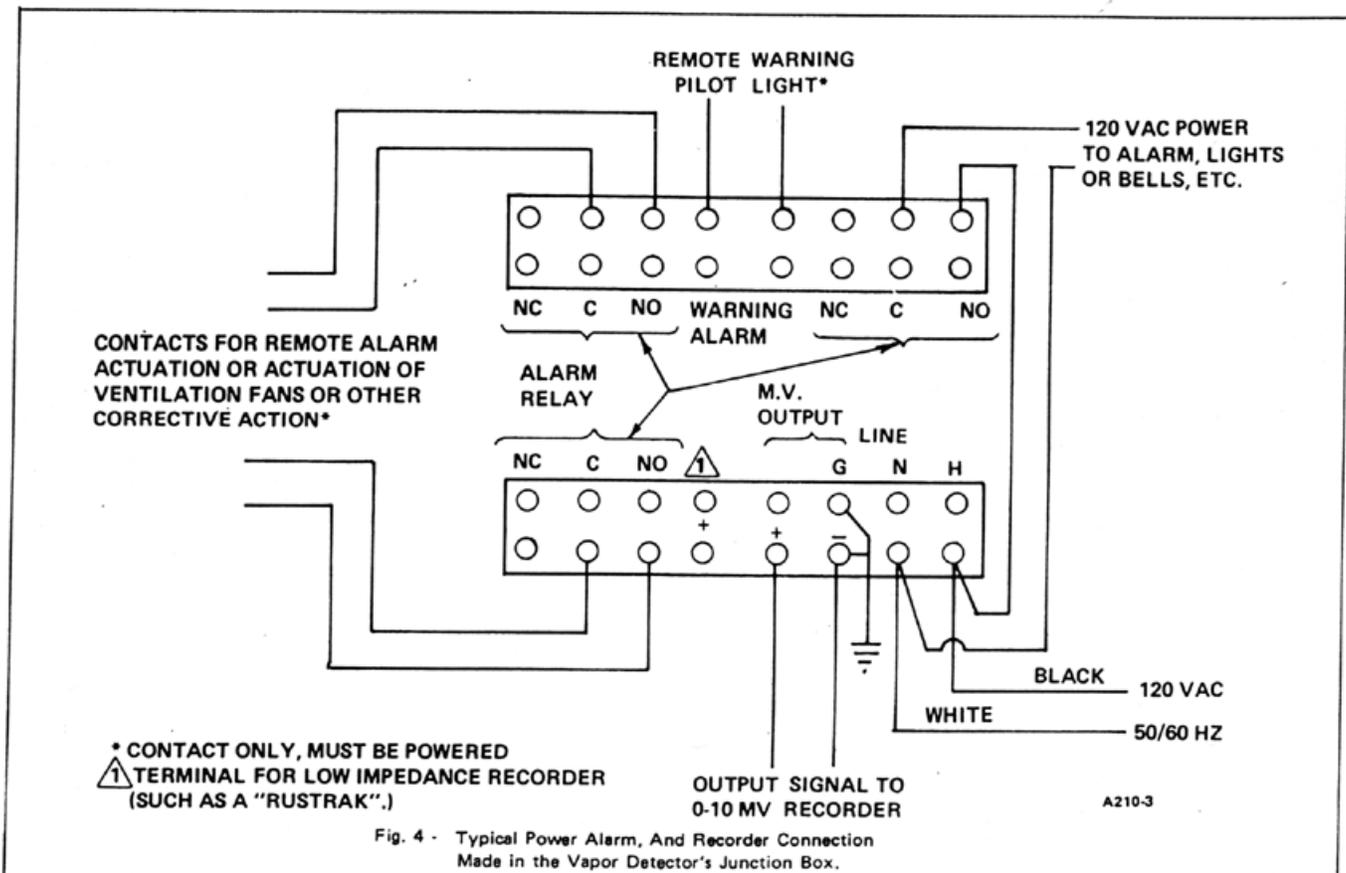
Fig. 4 - Typical Power Alarm, And Recorder Connection Made in the Vapor Detector's Junction Box.
