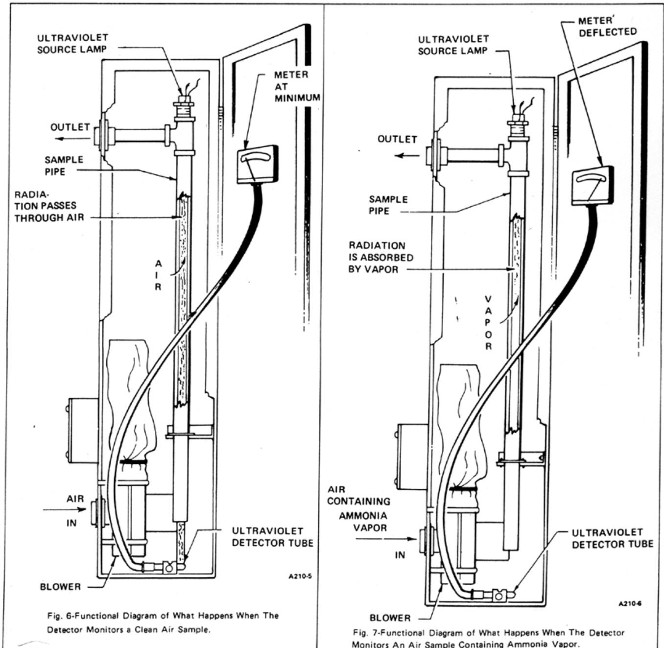
Fig. 6-Functional Diagram of What Happens When The Detector Monitors a Clean Air Sample.
